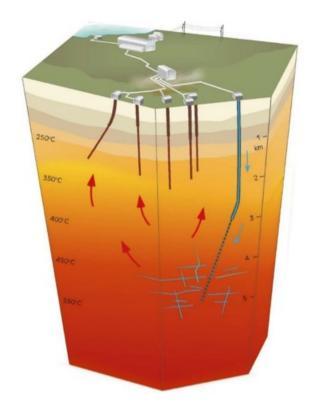
Figure 1: A conceptual model showing the EGS system in the Reykjanes field (Friedleifsson et al., 2016)
