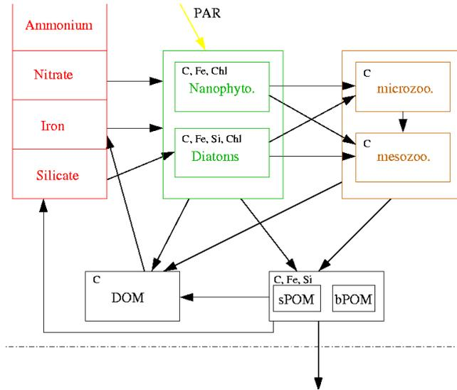
**Figure 1.** Architecture of PISCES. This figure only shows the ecosystem model omitting thus oxygen and the carbonate system. The elements which are explicitly modeled are indicated in the left corner of each box.
