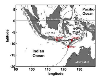
**Figure 1.** Map of the Indonesian seas showing pathways of the Indonesian Throughflow from the Pacific Ocean into the Indian Ocean. Lombok, Ombai, and Timor Straits are the major outflow passages of the ITF where moorings were located as part of INSTANT (red diamonds).
