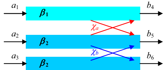
Fig. 2. Modelling of the directional coupler between the upper SMWG and the lower TMWG (itself seen as a set of 2 coupled SMWGs) as a six-port network; a_i = F_i(0) , b_j = F_j(d) .
