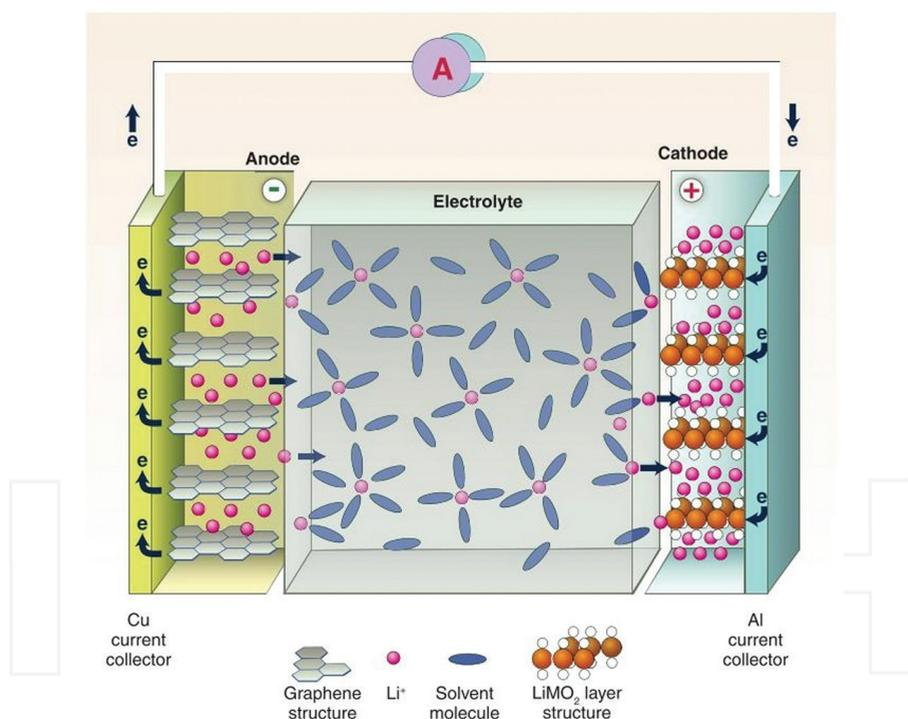
**Figure 1.** Schematic representation of the discharge of a  $\text{Li}^+$ -ion battery: a graphite-based negative electrode undergoes  $\text{Li}^+$  deintercalation, according to the following reaction:
