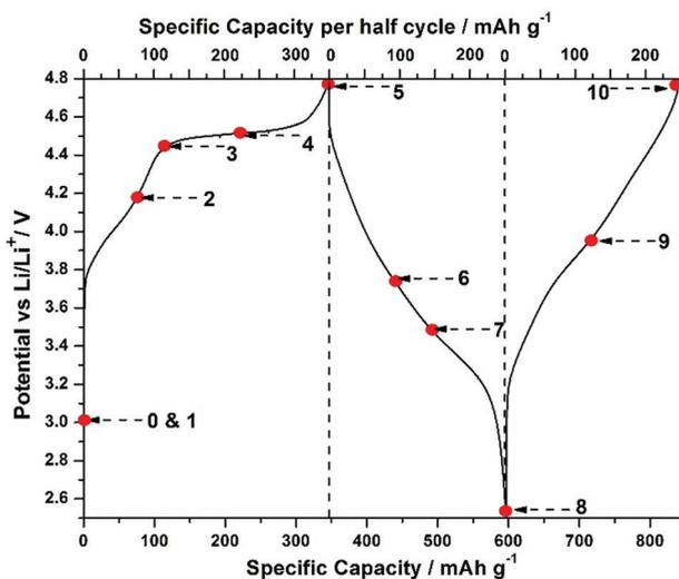
**Figure 5.** Voltage profile of two successive charge and discharge curves of Li-rich NCM at 20 mA/g. Representative points of 1–10 in the process of XAS measurements are indicated. Reference and counter electrode: Li. electrolyte: 1 M  $\text{LiPF}_6$  in EC/DMC. Temperature:  $20^\circ\text{C} \pm 2^\circ\text{C}$ . On the upper X axis the capacity detected in each step is reported. Reproduced from Ref. [54].
