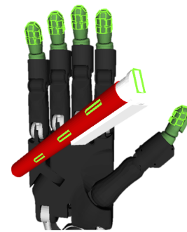
Fig. 16. The green spots are the predefined contact areas.
