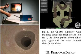
the force-torque feedback device (top left), the virtual patient colon editor (top right) and the colon internal
