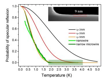
FIG. 4. Extracted probability of specular reflection for the nanowire (light green) and the narrow microwire (dark green) in comparison to the theoretical fit from Ziman approach using Eq. 5 with different roughness. The hatched area shows a purely diffusive regime known as the Casimir regime where the MFP becomes equal to the diameter of the nanostructure. In inset, an SEM picture of the SiN nanowire edge is shown. The actual roughness is much smaller than 9 nm.
