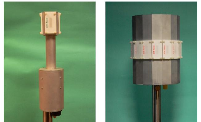
Fig. 1. UCA 4-elements transmitter (left) and 16-elements receiver (right).
