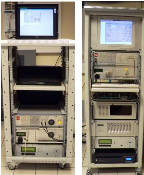
Fig. 3. MIMO channel sounder: Transmitter (left) and receiver (right).
