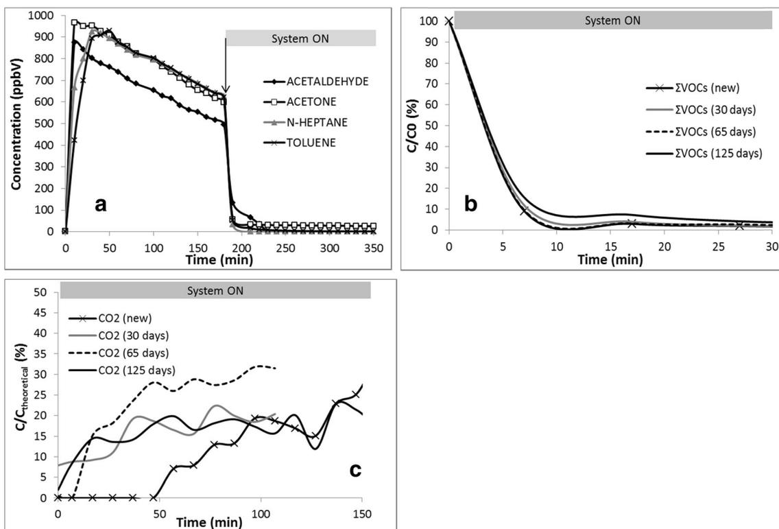
**Fig. 2** Examples of results according to XP-B44-013 standard with the photocatalytic air purifier E15. **a** Evolution of the concentration of individual VOC with time. **b** Drop of total VOC concentration. **c** Evolution of
