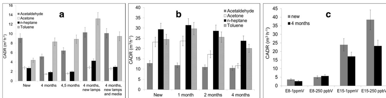
**Fig. 4** Influence of system ageing (system continuously switched on in the laboratory during the time indicated on the x axis) on the calculated CADR on individual VOC (standard XP-B44-013, each pollutant
