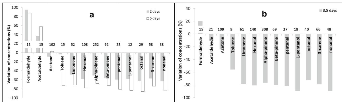
**Fig. 6** Evolution of VOC concentration with the two most efficient photocatalytic air-purifiers **a** E8 switched ON for 2 and 5 days; **b** E15 (4 months aging) switched ON for 3.5 days in the experimental platform BEF. The numbers on the bars are the initial VOC concentration ( $\mu\text{g m}^{-3}$ )
