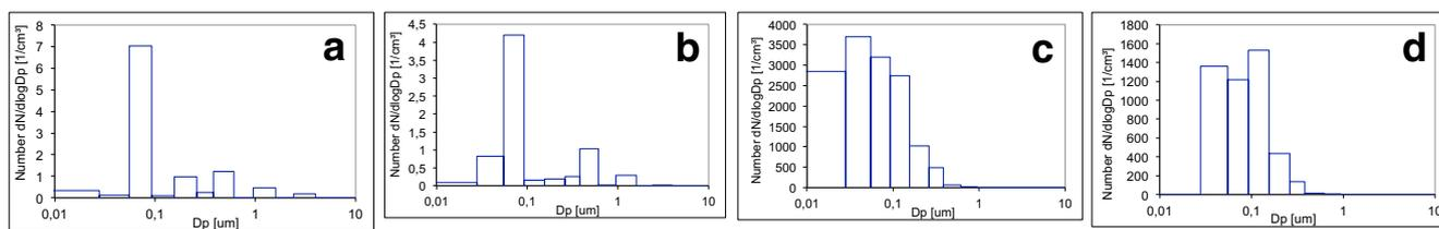
**Fig. 8** Measurements of micro/nanoparticles by ELPI. **a** control blank inside the flushed airtight chamber, **b** inside the airtight chamber with E15 ON for 4 h, **c** control outside the BEF platform, **d** inside the BEF platform with E15 ON after 30 days of continuous run, measured the same days as **c**
