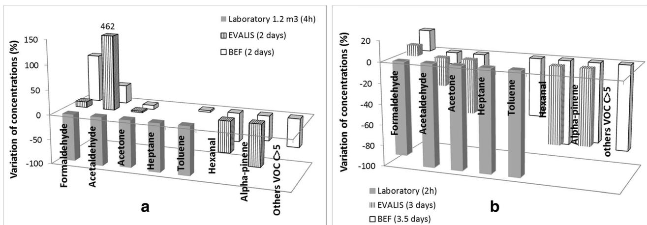
**Fig. 7** Evolution of VOC concentration with the two most efficient photocatalytic air purifier **a** E8 (number 462 was added on the bar because it was out of scale), **b** E15 in the airtight chamber or in experimental platforms EVALIS and BEF
