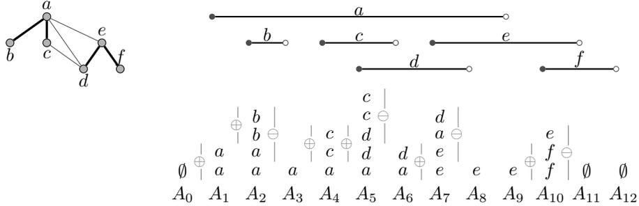
Figure 4: Left: An interval graph with six vertices and a  $P_3$ -partition  $\mathcal{P}$  (bold). Right: Interval representation of this graph and successive token lists  $A_0, \dots, A_{12}$  computed by Algorithm 1 (additions and deletions are marked with  $\oplus$  and  $\ominus$ ).
