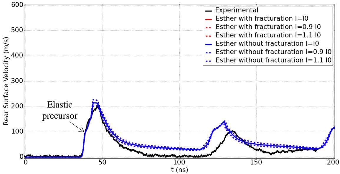
**Fig. 6** Rear Surface velocity profile obtained by simulation (+/- 10% on E) with fracturation (red) and without fracturation (blue) and compared to the experimental signal – Aluminum 6061 –  $E=6.1 \text{ J}$  –  $t=250 \text{ }\mu\text{m}$  –  $\tau=10 \text{ ns}$  –  $d_{\text{foc}}=1 \text{ mm}$  ( $I=50 \text{ GW/cm}^2$ )
