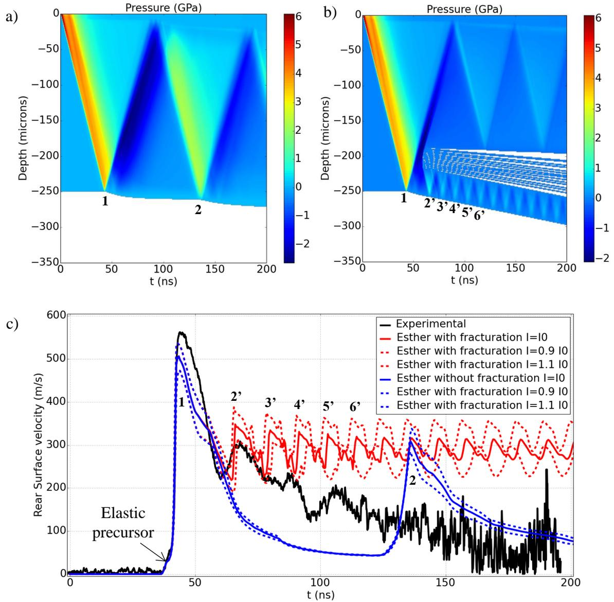
**Fig. 3** Space-time diagram without fracturation model (a), with fracturation model (b) and rear surface velocity profile (c) obtained by simulation (+/- 10% on E) with fracturation (red), without fracturation (blue), and compared to the experimental signal – Pure Aluminum –  $E=18.3 \text{ J}$  –  $t=250 \text{ }\mu\text{m}$  –  $\tau=10 \text{ ns}$  –  $\text{dfoc}=1 \text{ mm}$  ( $I=170 \text{ GW/cm}^2$ )
