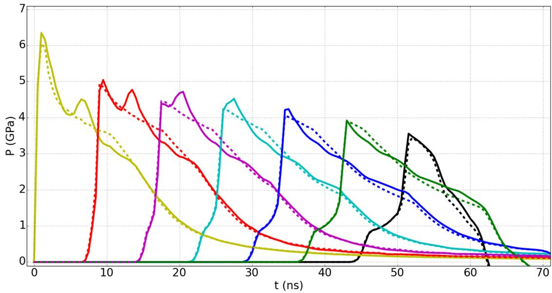
**Fig. 8**  $P_{abl}(t)$  (yellow) and  $P(t)$  at 50  $\mu\text{m}$  (red), 100  $\mu\text{m}$  (magenta), 150  $\mu\text{m}$  (pale blue), 200  $\mu\text{m}$  (dark blue) and 250  $\mu\text{m}$  (green) of propagation for a 10-ns GCLT Top-Hat (full lines) and 10-ns numerical  $F_{eq}$  Top-Hats (dotted line)
