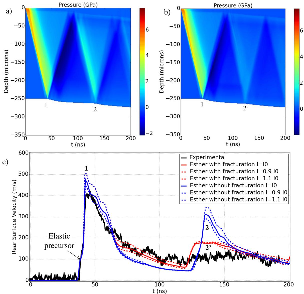
**Fig. 4** Space-time diagram without fracturation model (a), with fracturation model (b) and rear surface velocity profile (c) obtained by simulation (+/- 10% on E) with fracturation (red), without fracturation (blue), and compared to the experimental signal – Aluminum 6061 –  $E=20.3 \text{ J}$  –  $t=250 \text{ }\mu\text{m}$  –  $\tau=10 \text{ ns}$  –  $d_{\text{foc}}=1 \text{ mm}$  ( $I=180 \text{ GW/cm}^2$ )
