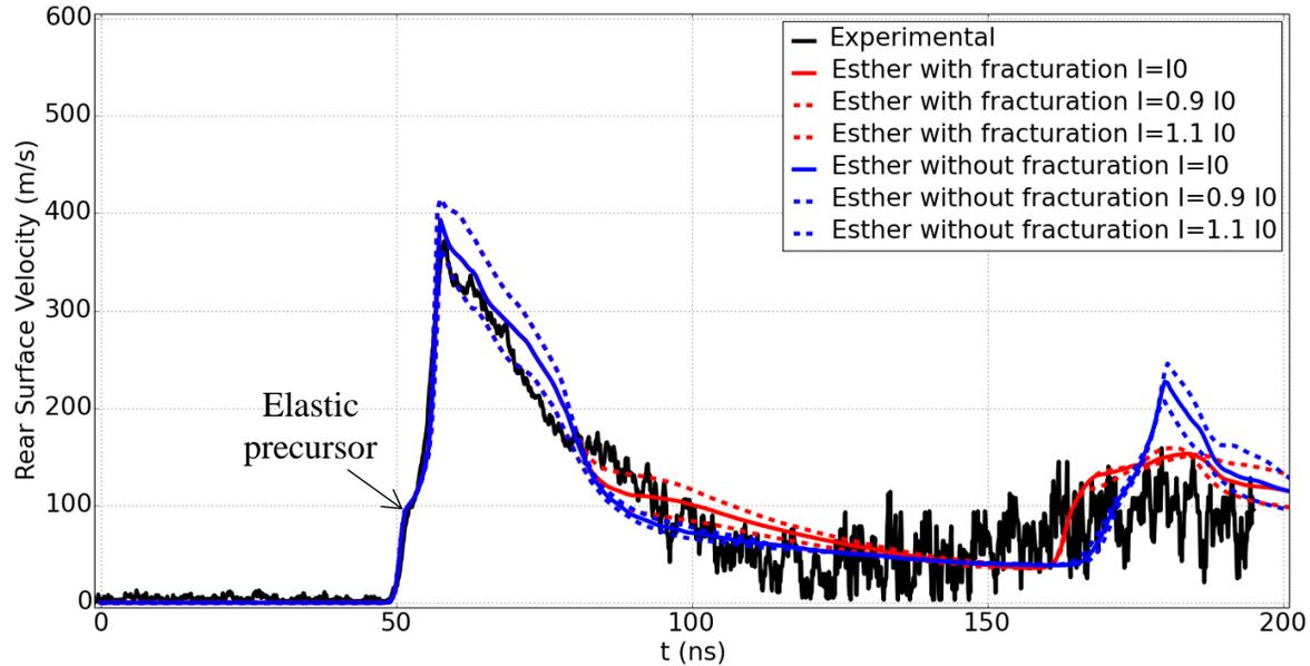
**Fig. 5** Rear surface velocity profile obtained by simulation (+/- 10% on E) with fracturation (red) and without fracturation (blue) and compared to the experimental signal – Aluminum 6061 –  $E=18.2 \text{ J}$  –  $t=335 \text{ }\mu\text{m}$  –  $\tau=10 \text{ ns}$  –  $d_{\text{foc}}=1 \text{ mm}$  ( $I=170 \text{ GW/cm}^2$ )
