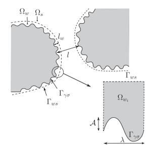
**Fig. 2.** Schematics of the multi-domain decomposition.  $\Gamma_{ws}$  and  $\Omega_s$  refer to the effective surface and domain, respectively.  $\Omega_w$  is the subdomain that contains the rough wall and  $\Omega_{w_l}$  is the local domain over a rough element.  $l_w$  is the characteristic distance from the rough pattern to the effective surface and l is the characteristic length scale of the pore. A and  $\lambda$  are the amplitude and wavelength of the roughness.
