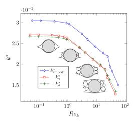
**Fig. 8.** Dimensionless apparent permeability  $k^*$  along the *x*-axis as a function of the Reynolds number for the effective condition  $k_s^* = \frac{k_s^*}{d^2}$ , the rough  $k_{\gamma}^* = \frac{k_s^*}{d^2}$  and smooth  $k_{smooth}^* = \frac{K_{mooth}}{d^2}$  cylinders.
