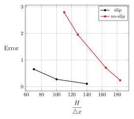
**Fig. 19.** Plot of the error as a function of the average number of mesh elements per direction,  $\frac{H}{\Delta x^{\epsilon}}$  The error is defined  $100\left(\left\|\frac{|(u_{k})-(u_{k})|_{R}}{(u_{k})|_{R}}\right\|\right)$  where  $\langle u_{x} \rangle|_{R}$  is a reference average velocity obtained with an extremely fine mesh,  $\frac{H}{\Delta x} = 180$  for the smooth surface and  $\frac{H}{\Delta x} = 285$  for the rough surface
