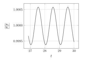
**Fig. 12.** Volume averaged velocity  $\langle \mathbf{u}_s \rangle$  as a function of time for  $Re_k = 29$  ( $Re_d = 168$ ).
