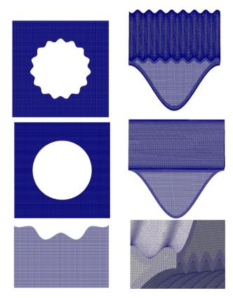
**Fig. 20.** Meshes for the unit-cell of the array of beads (left) and for the element of packings (right). Domains  $\Omega_{\gamma}$  and  $\Omega_s$  are given. The element of packings corresponds to the geometry *a*.
