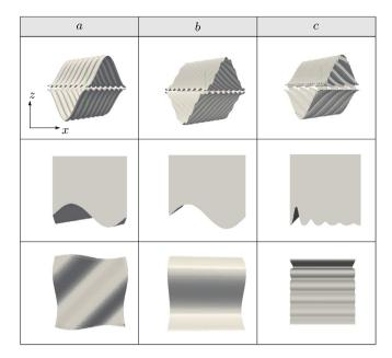
**Fig. 14.** Geometries considered in the simulations. The first line shows the unitcells of structured packings, while the second and third lines are the rough elements  $\Omega_{w_i}$  on the surface. Roughness types *a* and *b* correspond to typical wall-textures that can be engineered on the surface. Roughness *c* represents a traveling train of soliton waves along the column axis.
