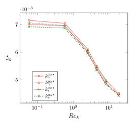
**Fig. 18.** Dimensionless permeability  $k^*$  coefficients in the *x* and *y* directions as functions of the Reynolds number for the geometry *b*. Results show good agreement between the exact and effective permeabilities with the anisotropy  $k_s^{xx*} > k_y^{yy*}$ .
