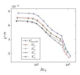
**Fig. 16.** Dimensionless permeability  $k^{\star,yy}$  along the *y*-axis for the geometries *a* and *c* as a function of the Reynolds number. The exact permeabilities of the smooth  $k_{smooth}^{\star} = \frac{K_{tmoth}^{\star}}{H^2}$  and rough  $k_{\gamma}^{\star} = \frac{K_{\tau}^{\star}}{H^2}$  domains are compared to the permeability  $k_{s}^{\star} = \frac{K_{\tau}^{\star}}{H^2}$  obtained with the tensorial slip condition.
