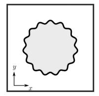
Fig. 7. Illustration of a unit-cell for a 2D array of rough cylinders.
