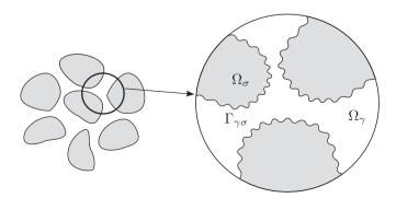
**Fig. 1.** Schematics of a porous medium with rough walls.  $\Omega_{\sigma}$  and  $\Omega_{\gamma}$  are, respectively, the solid and fluid phases.  $\Gamma_{\gamma\sigma}$  is the rough surface of the porous medium.
