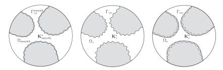
Fig. 4. Schematics of the different domains considered for comparison.  $K_{smooth}^{\star}$ ,  $K_{\gamma}^{\star}$  and  $K_{s}^{\star}$  are, respectively, the permeability in the smooth, rough and effective domains.
