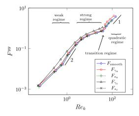
**Fig. 17.** Correction coefficient along the *y*-axis  $F^{yy}$  for the geometries *a* and *c* as a function of the Reynolds number. The exact corrections of the smooth  $F_{\text{smooth}}$  and rough  $F_{\gamma}$  domains are compared to the correction  $F_s$  obtained with the tensorial slip condition.
