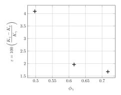
**Fig. 13.** Error between exact and effective intrinsic permeabilities for three porosity levels. Cylinder diameters from left to right: d/H = 0.8,  $(l_w/l = 0.0250) d/H = 0.7$ ,  $(l_w/l = 0.0167)$ , and  $d/H = 0.6 (l_w/l = 0.0125)$ .
