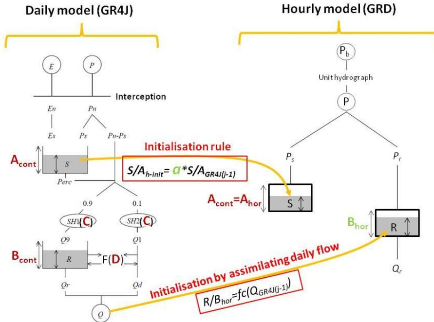
**Fig. 2.** The coupling between the daily model (GR4J) and the hourly model (GRD), with the 2 initialisation rules (production and routing, in red) and the parameters to be calibrated (4 GR4J parameters in dark red, and 2 GRD parameters in green).
