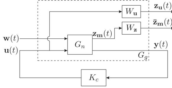
Fig. 2. Block diagram of the  $H_\infty$  control problem.
