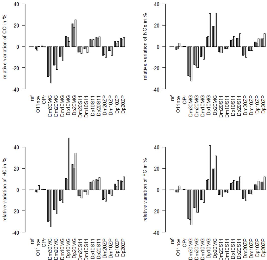
Figure 2: relative variation of the environmental parameters calculated for each scenario to the reference scenario. The darker grey: Copert, medium grey: HBEFA, light grey: Phem estimations.
