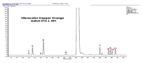
Total Ion Current profile of the impurities present in the batch #5 of the Vibracolor Copper Orange colorant using the Total Ion Current detection (FT-ICR)
