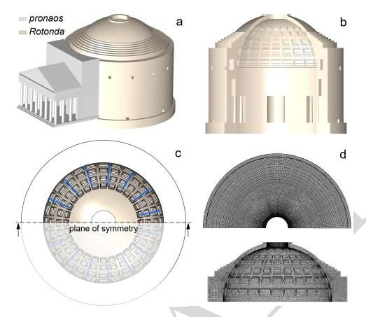
Figure 14: The model of the Pantheon; a) overall view, b) interior view of the *Rotonda*, c) detail of the dome with indicated the meridional cracks inserted in the model, and d) details of the structural mesh MS11.
