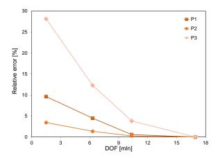
Figure 12: Relative error, eq. (15), for points P1 to P3 as function of the number of DOF.
