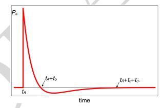
Figure 4: Scheme of the time variation of the pressure due to a blast.
