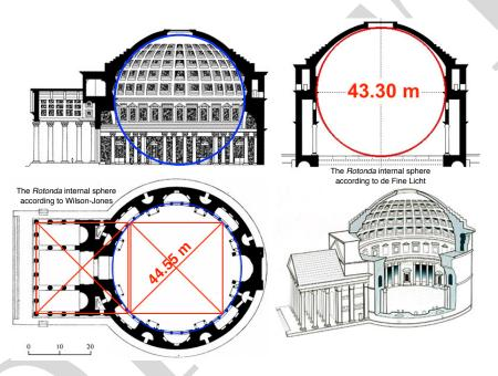
Figure 2: Scheme and dimensions of the Pantheon (from [Pulvirenti, 2014]).
