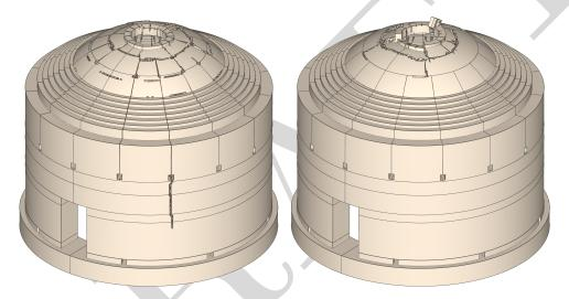
Figure 22: Comparison of the structural damage of the dome at the end of the calculations: with pre-existent cracks (left) and without (right).
