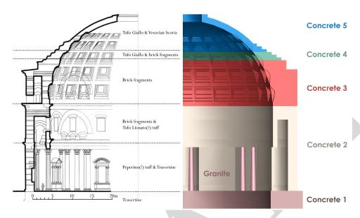
Figure 5: Materials composing the *Rotonda* as in [Lancaster, 2005] (left) and as in Tab. 3.
