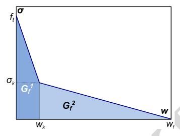
Figure 8: Traction-separation diagram and fracture energy.
