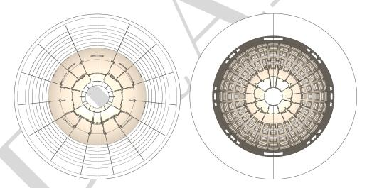
Figure 19: Structural damage of the dome at the end of the calculations: external (left) and internal (right) views.
