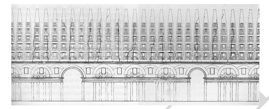
Figure 3: Meridional cracks in the *Rotonda's* dome (after [Terenzio, 1934]).
