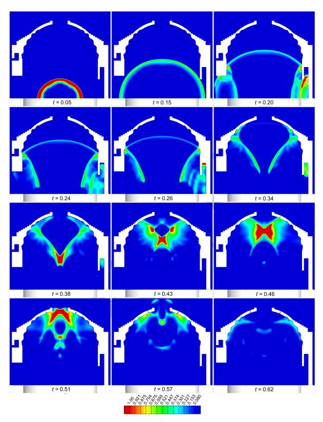
Figure 17: The evolution of the (normalized) overpressure field inside the *Rotonda*. Dark blue regions represent negative or zero overpressure.
