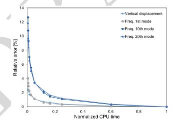
Figure 16: Relative error versus the normalized CPU time.
