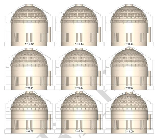
Figure 20: The evolution of the structural damage of the *Rotonda*, without pre-existent cracks.
