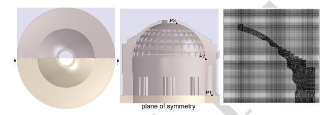
Figure 10: The air domain: overall view and location of the observation points P1 to P3 (left) and detail of the mesh (right).
