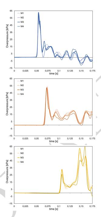
Figure 11: Time history of the overpressure for points P1 to P3 (from top to bottom).
