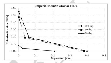
Figure 7: Best-fit traction-separation descriptions for each curing duration, according to [Brune, 2010].
