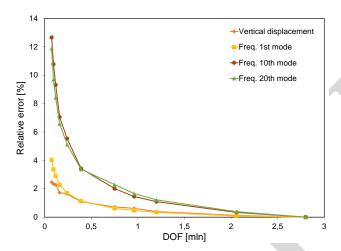
Figure 15: Relative errors  $\Delta f_1$ ,  $\Delta f_{10}$ ,  $\Delta f_{20}$  and  $\Delta u$  as function of the number of DOF.
