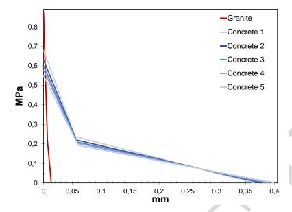
Figure 9: Traction-separation diagram of the materials composing the Pantheon.
