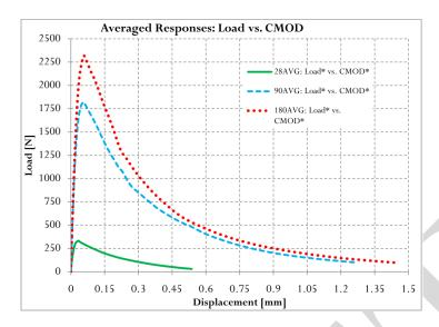
Figure 6: Average characteristic response for different curing times, according to [Brune, 2010].
