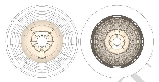
Figure 21: Structural damage of the dome at the end of the calculations: external (left) and internal (right) views, without pre-existent cracks.
