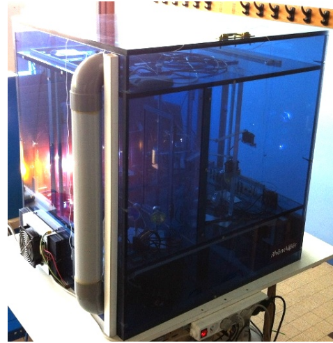
Figure 1: Small-scale experiment of a flat with UFAD regulation
