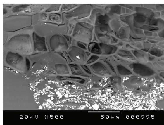
Figure 8 Back-scattered electron micrograph of a cross-section of the paper pulp (sampled in left hip) showing polygonal cells which were identified as cork cells. © Inp / M.-C. Papillon.
