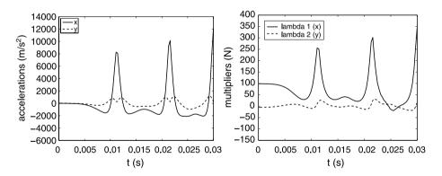
Fig. 7 (x, y)-accelerations of point P and Lagrange multipliers
