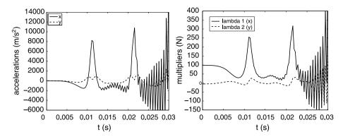
**Fig. 8** Without numerical damping: (x, y)-accelerations of point P and Lagrange multipliers associated with the (x, y) internal forces in body 1
