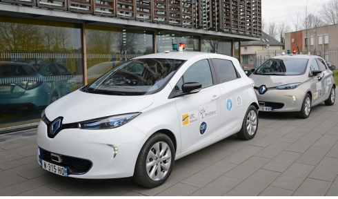
Fig. 6. ApACHE autonomous electric cars. The white vehicle is leading the way while the gray one is platooning.
