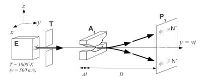
Figure 1: Schematic configuration of the historic Stern-Gerlach experiment: a beam of silver atoms [4], from the source (oven **E**, collimator hole **T**) passes through an inhomogeneous magnetic field (magnet  $A_1$ ), then separates into two distinct beams before condensing on the screen  $P_1$  on two distinct spots of identical intensity  $N^+$  et  $N^-$ .
