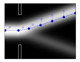
Figure 8: dBB theory (quantum mechanics taken one step further): Pauli equation + initial position. The arrows indicate the  $\theta$  orientation of the spin vector s (initially  $\theta_0 = \pi/3$ ). The position of the particle exists before the measurement; the particle follows a deterministic trajectory and the impact on the screen only reveals its position. The atom is both a wave *and* a particle during all the experiment.
