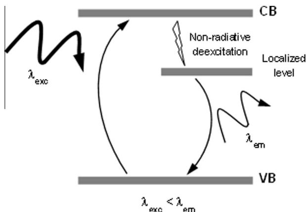
**Fig. 1.** The mechanism of the down-shifting process; VB is the valence band, CB - the conduction band,  $\lambda_{exc}$  is the excitation wavelength; non-radiative deexcitation to the localized level in the bandgap via the emission of phonons is shown; the radiative emission from the intermediate energy level at the  $\lambda_{em}$  wavelength follows the excitation.
