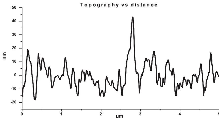
Fig. 3. The AFM image and the topography of the  $\text{ZnO}_x$  nanoparticle layer deposited by the LECBD technique on the top of an Si solar cell.
