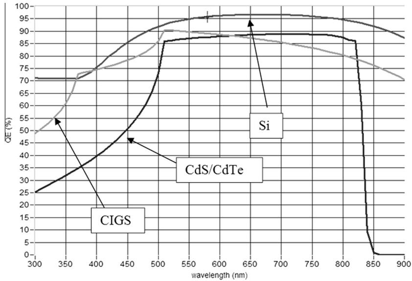
**Fig. 4.** Numerical SCAPS simulation of external quantum efficiency (marked as QE in the graph) for a standard Si cell (dark grey curve), the CIGS cell (light grey curve) and the CdTe cell (black curve) in function of the incident solar light wavelength.
