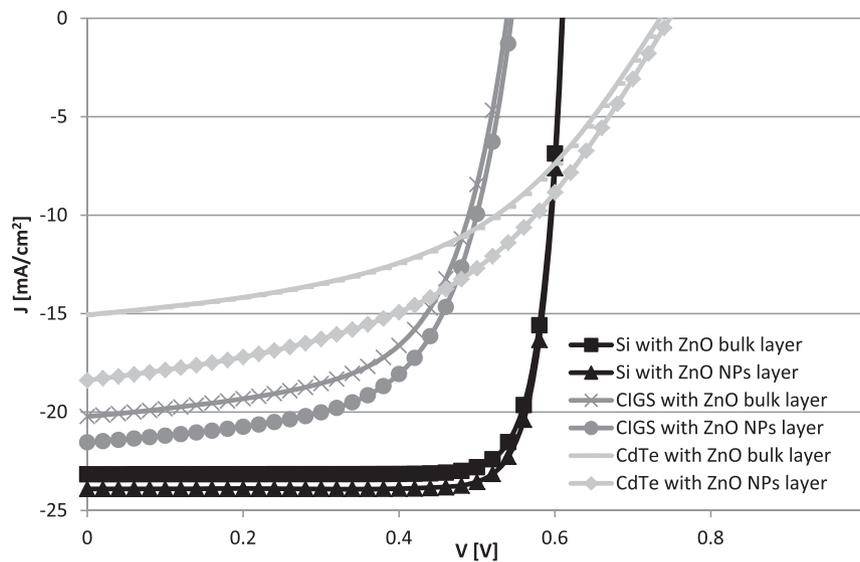
Fig. 7. The simulations of the  $I$ - $V$  characteristics obtained using the SCAPS program of the Si, CIGS and CdTe solar cells with ZnO passive antireflective layer (marked as “with ZnO bulk layer” in the legend) or with a  $ZnO_x$  NPs down-shifting layer (marked as “with ZnO NPs layer” in the legend) on their top, under AM 1.5 G illumination.
