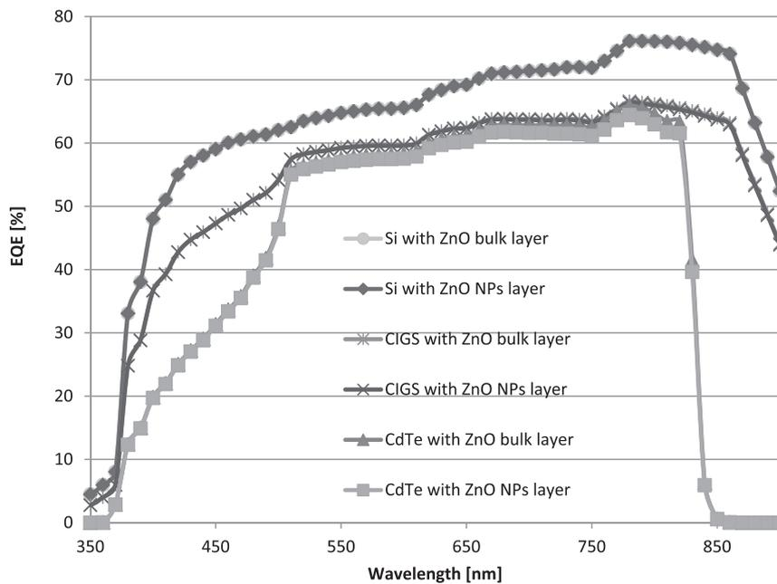
**Fig. 5.** EQE characteristics simulated using the SCAPS program of the Si, CIGS and CdTe solar cells, covered or by a bulk ZnO passive antireflective layer (marked as “with ZnO bulk layer” in the legend) or by a ZnO<sub>x</sub> NPs LDSL (marked as “with ZnO NPs layer” in the legend), taking into account the modification of the solar illumination spectrum by the presence the DS layer in the structure of the cell.
