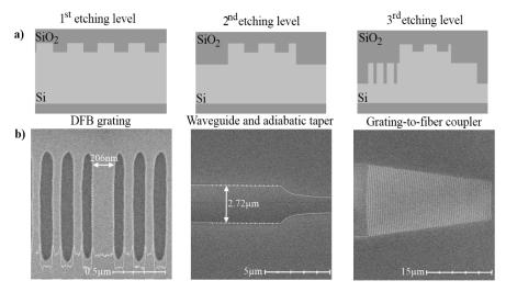
Fig. 5. (a) Schematic side views of the Si waveguide for the first three etching levels: the DFB grating, the rib waveguide with the adiabatic taper and the grating-to-fiber coupler (b) Corresponding top SEM view after each etching.
