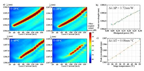
Fig. 9. (a) Laser spectra as a function of the pumping current for various stage temperatures:  $25^{\circ}$ C,  $35^{\circ}$ C,  $45^{\circ}$ C and  $55^{\circ}$ C Laser peak wavelength as a function of the dissipated power (CW) (b) as well as of the stage temperature in pulsed regime (c).
