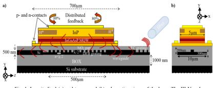
Fig. 1. Longitudinal (a) and transversal (b) schematics views of the laser. The III-V and the silicon waveguide are separated by a  $SiO_2$  gap of 75nm. The DFB grating is etched along the silicon waveguide underneath the III-V active layers. The active region consists in InGaAsP multiple QWs surrounded by *p*- and *n*-doped InP layers.
