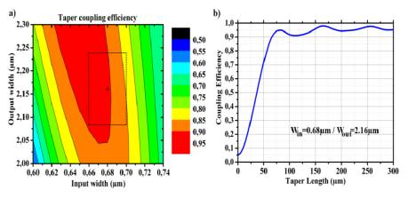
Fig. 3. (a) Taper coupling efficiency depending on the input and output width of the rib silicon waveguide. The cross represents the dimensions chosen and the dashed square stands for the process variation window. (b) Taper coupling efficiency as a function of the taper length with  $W_{in} = 0.68 \mu m / W_{out} = 2.16 \mu m$ .
