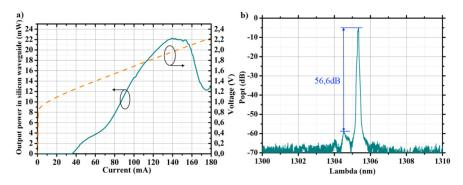
Fig. 8. Room-temperature LIV (a) and spectrum of the laser at I = 107mA (b). The resolution of the optical spectrum analyser (OSA) was 0.02 nm.
