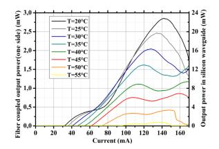
Fig. 7. *L-I* curves with increasing temperature. The left scale gives the output power in the fiber while the right scale gives the output power obtained in the waveguide.
