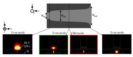
Fig. 2. Schematic top view of the adiabatic taper in the silicon rib and electric field distributions (|E|) at the input, output and middle of the taper for the even mode. The odd mode is represented at the middle: the taper is designed to get rid of this mode and have all the power in the even mode.
