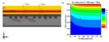
Fig. 4. (a) Schematic side view of the grating underneath the III-V active region with the  $\lambda/(4n_{eff})$  defect in the middle of the grating. The modal repartition is represented when the Si waveguide is or is not etched. (b) Grating coupling constant ( $\kappa_r$ ) calculated values. The cross represents the  $\kappa_r$  of our design (25.5 cm<sup>-1</sup>).
