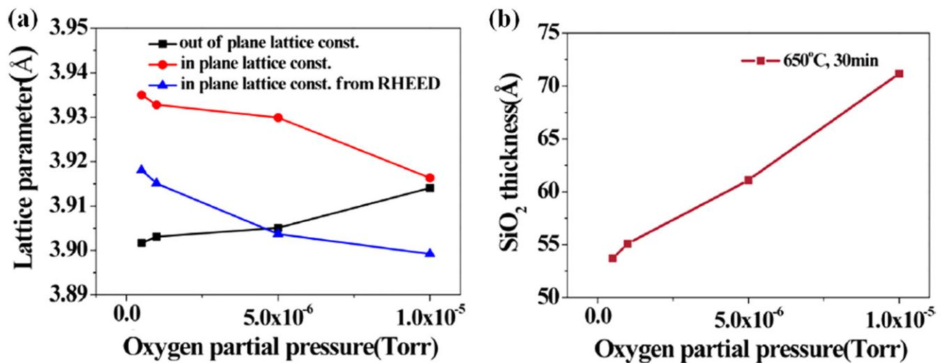
**Figure 2.** (a) In-plane and out-of-plane lattice constants and (b) SiO<sub>2</sub> thickness as a function of oxygen partial pressure. All films were annealed at 650 °C for 30 min in different oxygen environments. From figure 5 in [96]. Reprinted with permission from M Choi *et al* 2012 *J. Appl. Phys.* **111** 064112. Copyright 2012, AIP Publishing LLC.
