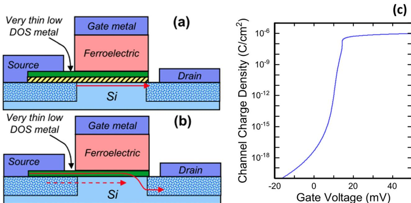
**Figure 8.** Device structures for FeFET with quantum metal layer. The arrows indicate current flow paths. (a) With and (b) without a thin insulator between the quantum metal and the semiconductor—(c) calculated  $Q$ - $V$  curve for an FeFET as represented in (a)—DOS stands for ‘density of state’. Adapted from figures 4 and 6(a) in [178]. Reprinted with permission of IEEE (D Frank *et al* 2014 *IEEE Trans. Electron Devices* 61 2145).
