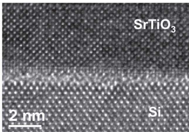
**Figure 1.** High-resolution TEM image of a SrTiO<sub>3</sub> thin film deposited on Si (001) substrate by MBE.
