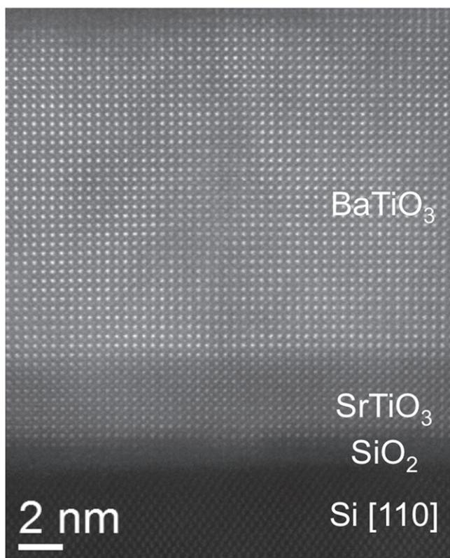
**Figure 6.** Scanning transmission electron microscopy high-angle annular dark field (HAADF) image of a BaTiO<sub>3</sub>/SrTiO<sub>3</sub> stack grown on Si (001), indicating a sharp interface between SrTiO<sub>3</sub> and BaTiO<sub>3</sub> and a high crystalline quality of the perovskite oxides.
