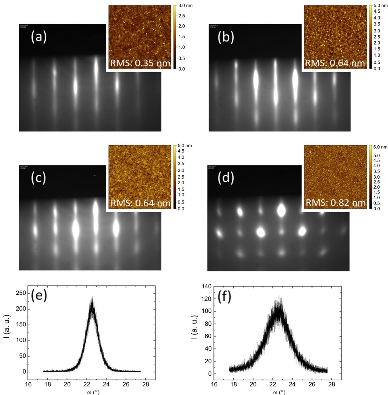
**Figure 4.** (a)–(d) RHEED patterns recorded along the [100] azimuth during BaTiO<sub>3</sub> growth at 450 °C under an oxygen pressure of (a)  $1 \times 10^{-7}$  Torr, (b)  $5 \times 10^{-7}$  Torr, (c)  $2 \times 10^{-6}$  Torr, (d)  $3 \times 10^{-6}$  Torr and corresponding AFM images of the film surfaces. (e)–(f) Rocking curve measured on the 002 peak for the films grown at (e)  $5 \times 10^{-7}$  (FWHM = 1.5°) and (f)  $2 \times 10^{-6}$  Torr (FWHM = 2.9°).
