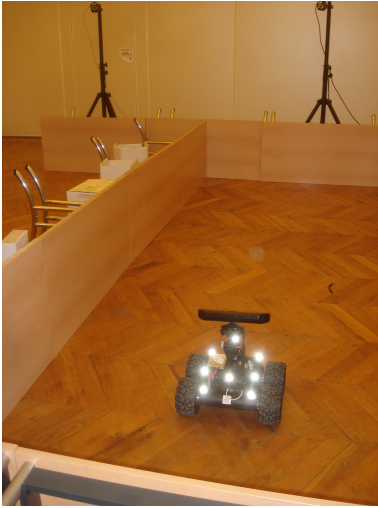
Fig. 1. Testing arena with Wifibot robot in the foreground of the picture. We can also see two of the seven Optitrack cameras in the background.
