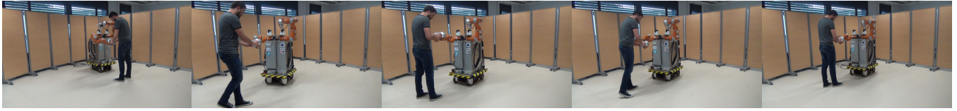
(a) Base is fixed, arm is moving. t < 12s (b) Base is moving, arm is fixed. 12s < t < 30s (c) Base is fixed, arm is moving. 30s < t < 38s (d) Both base and arm are moving. 38s < t < 47s (e) Base is fixed, arm is moving. t > 47s
