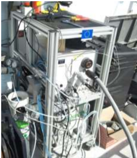
Figure 1: Gas analysers on-board a cargo vessel; sampling (heated line) and concentration measurement
