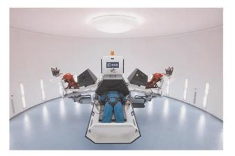
**Figure 4.** European Space Agency short-arm human centrifuge at DLR (Cologne). Maximum radius at outer perimeter: 2.8 m; maximum centrifugal acceleration: 4.5 g (foor level, test subject height: 1.85 m); number and type of nacelles: two beds, two seats; maximum overall payload: 550 kg (Credit ESA and DLR).
