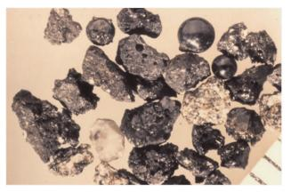
**Figure 6.** Lunar dust is covered in a glassy coating that can either be smooth or jagged (Credit: Larry Taylor).
