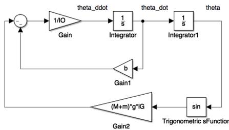
Fig. 3: Simulink model for the rotational pendulum
