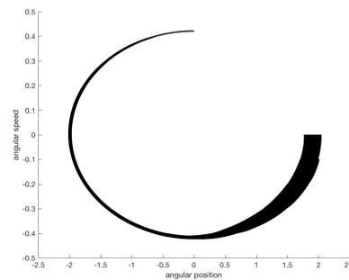
Fig. 7: Reachability results of the rotational pendulum for a global time horizon of 1s. Phase portrait of the angular position (rad) and angular speed (rad/s).
