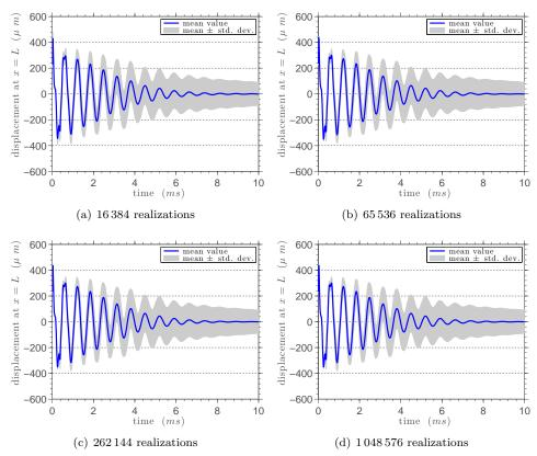
Figure 5. This figure illustrates the mean value (blue line) and a confidence interval (grey shadow) with one standard deviation, of the random process  $U(L,\cdot,\cdot)$ , for several values of MC realizations.
