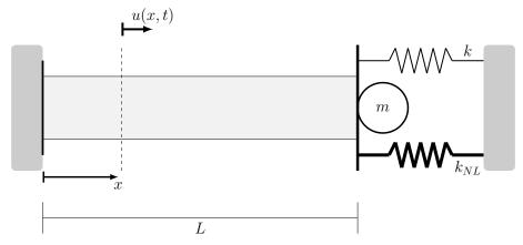
Figure 2. Sketch of a bar fixed at one and attached to two springs and a mass on the other extreme.
