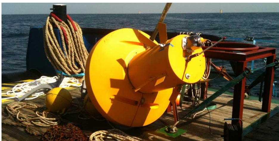
Real-time underwater noise monitoring buoy to be deployed in German Offshore WindFarm – picture credits Baker Consultants
