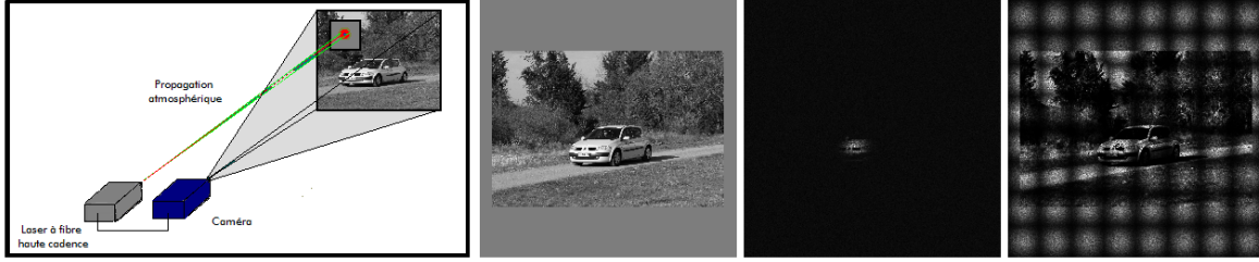
Figure 1. Left to right: the mosaic laser imaging process, the ideal image we want to estimate, a reduced part of the field of view with a single laser flash, the image composed from all laser shots where each pixel is assigned with its maximum intensity over all of them.
