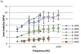
Figure 4. Storage (a) and loss (b) moduli for the three different phantoms and the two techniques, magnetic resonance elastography (dashed lines) and high-frequency rheometry (dotted lines). Results for phantoms (A), (B) and (C) appear in blue, green and orange, respectively.
