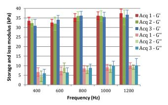
Figure 3. MRE results obtained for phantom A and three different acquisitions: Acquisition 1 is the reference acquisition; acquisition 2 was performed right after 1. Acquisition 3 was recorded ten days later.
