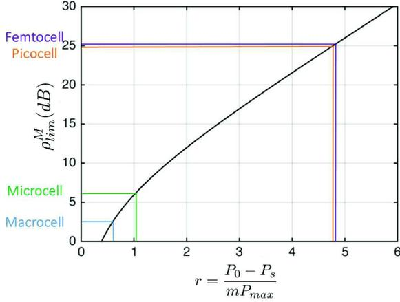
Fig. 2.  $\rho_{lim}^M$  versus  $r$ . This graph can be used to evaluate the value of  $\rho_{lim}^M$  for each BS type
