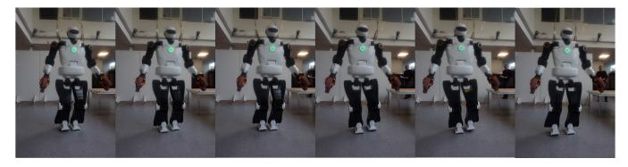
Fig. 9. Pyrène walking with bricks in both grippers. Each brick weight 1.5~Kg
