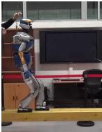
Fig. 2. (left) HRP-2 climbing dynamically stairs up to 15cm (right) HRP-2 walking on a beam.
