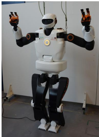
Fig. 1. Pyrene the first robot of the TALOS serie built by PAL-Robotics.
