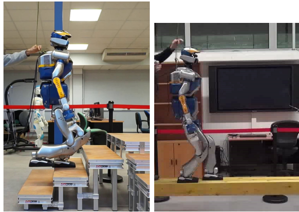
Fig. 2. (left) HRP-2 climbing dynamically stairs up to 15\text{cm} (right) HRP-2 walking on a beam.
