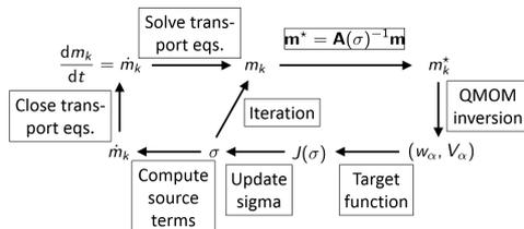
Figure 1: Schematic of the EQMOM algorithm.
