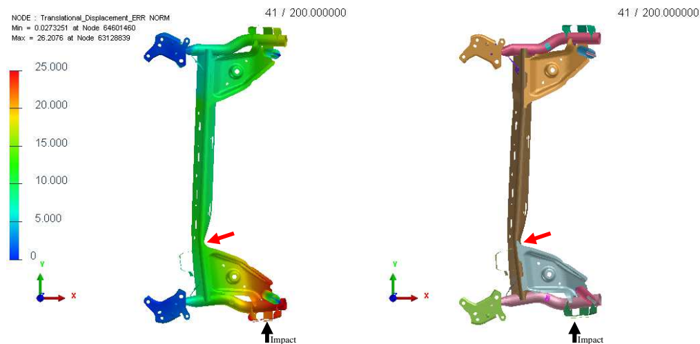
Figure 10: High-fidelity (VPS) calculation, right, and a reduced order model, left. On the reduced order model, nodal projection of the displacement error (%).
