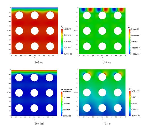
Figure 6: Visualization of the microcopic velocity and pressure with circular inclusions.
