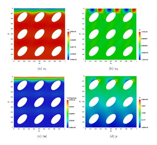
Figure 5: Visualization of the microcopic velocity and pressure with elliptical inclusions.
