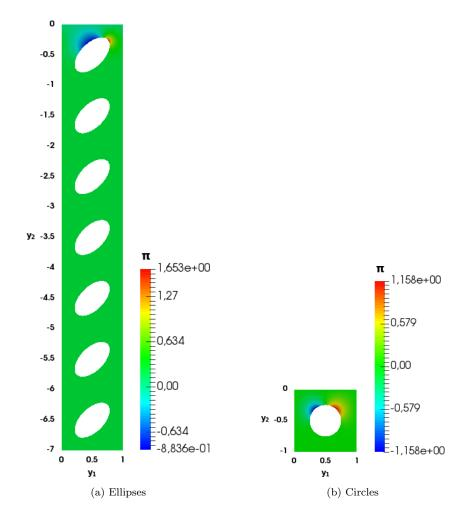
Figure 2: Visualization of boundary layer pressure and cut-off domain.
