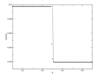
Figure 7: Fractional step method  $S_{FS}$  - 100 cells -Pure contact discontinuity. The continuous line refers to the exact solution. The initial data is given in section 5.2.1.
