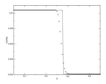
Figure 11: Fractional step method  $S_{FS}$ - 100 cells -Shock wave including void fraction desequilibrium. The initial data is given in section 5.2.3. The continuous line refers to the exact solution.  $T_{max} = 3.8729 \ 10^{-4}, \ \alpha_l(T_{max}) = 0.51039, \ \alpha_r(T_{max}) = 0.50208$
