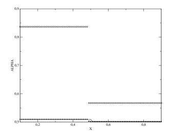
Figure 8: First and second cell schemes for Leroux method  $S_{UPW1}$ ,  $S_{UPW2}$  - 100 cells - The continuous line refers to the exact solution. The initial data is given in section 5.2.1.
