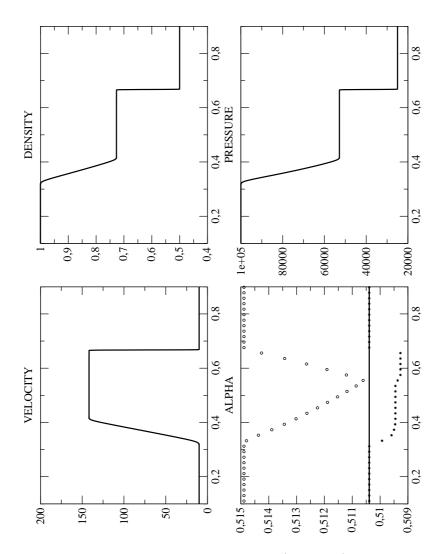
Figure 5: Numerical solutions for the shock tube test case (5000 cells) circles  $S_{UPW1}$ , black circles  $S_{UPW2}$ , continuous line  $S_{FS}$ . The exact solution cannot be distinguished from the current approximation obtained with  $S_{FS}$ .
