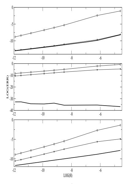
Figure 13: Convergence in  $L_1$  norm for  $\alpha - \tau_0 = 10^{-4}$ -Pure contact discontinuity, see section 5.2.1 (top) Shock wave with uniform void fraction profile, see section 5.2.2 (middle) Shock wave including void fraction desequilibrium, see section 5.2.3 (bottom) Symbols: circles  $S_{UPW1}$ , stars  $S_{UPW2}$ , continuous line  $S_{FS}$
