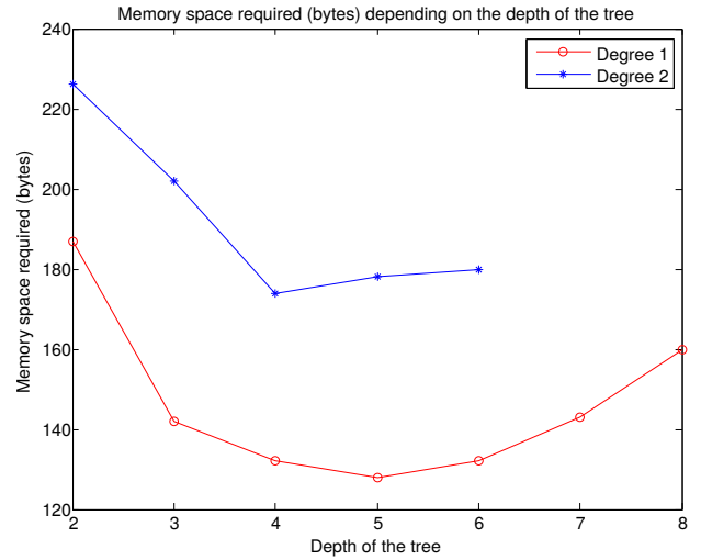
Fig. 8: Evolution of the memory space required to store the polynomials (table \mathcal{P} ) and the shifts (table \mathcal{D} ) (circles) and both polynomials ( \mathcal{P} ), shifts ( \mathcal{D} ) and the indexing table ( \mathcal{T} ) (diamonds) depending on N_l
