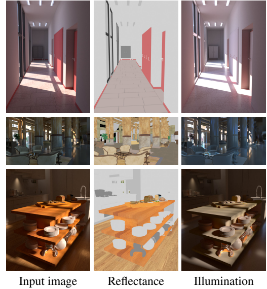
Figure 11: Three of our realistic ground-truth intrinsic decomposition results obtained with LuxRender [Ver07].
