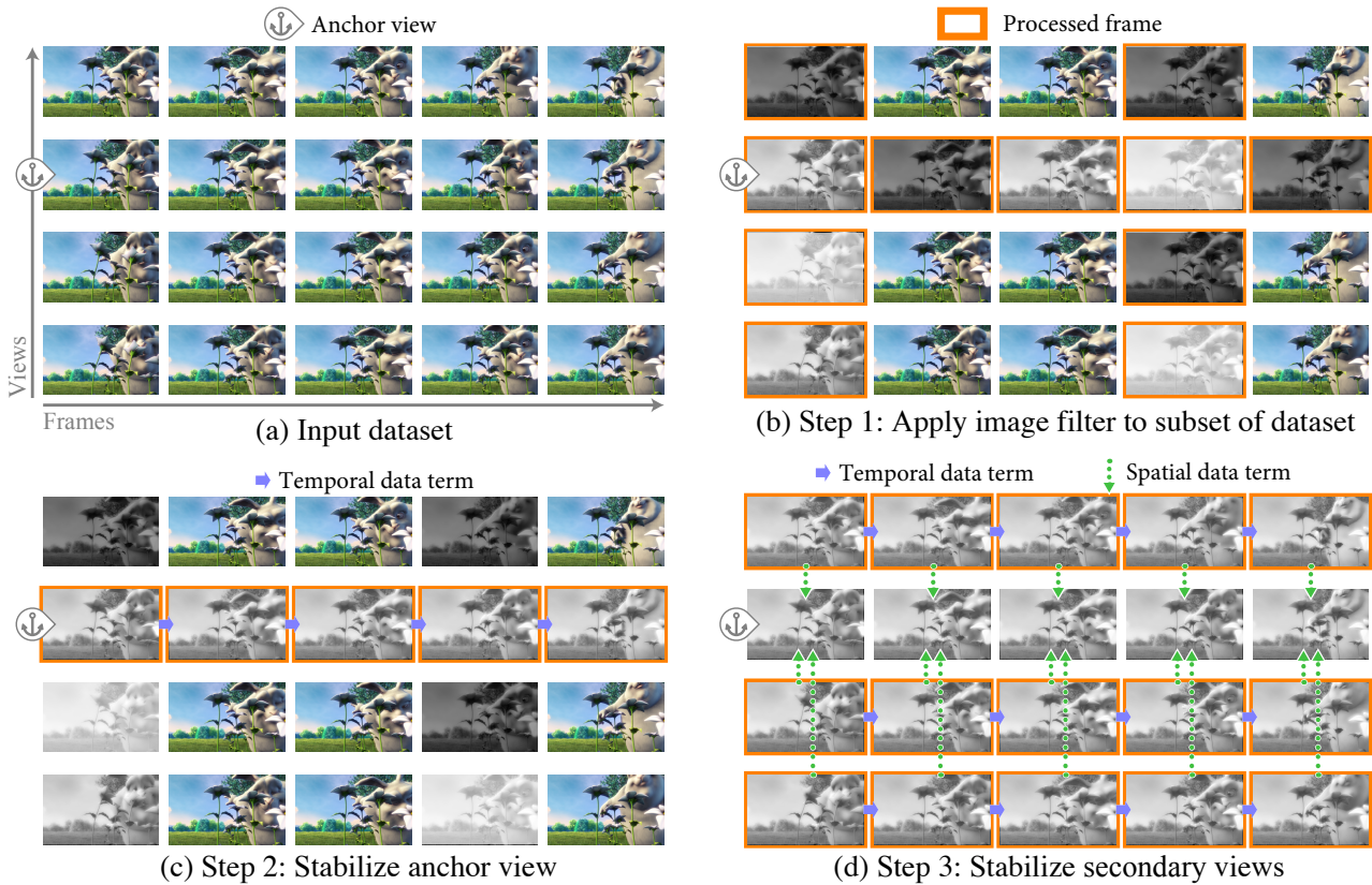
Figure 5: We accelerate our algorithm by applying image filter f only to a subset of the input data (a). We filter all frames at t = 0 and all anchor frames, and 1 in n frames for the secondary views (b). We use n = 3 in this example. The rest of the algorithm remains the same (c,d). This significantly speeds up the process while having a limited impact on the results because our algorithm is sufficiently robust to transfer the information from the filtered frames, essentially “hallucinating” the effect of the filter. We reorder this computation to be more storage efficient by interleaving (c) and (d) to create a streaming algorithm (§2.4). Please view in color. (‘Big Buck Bunny Flower’: \lambda_t = 0.1, \lambda_s = 0.1 .)
