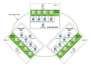
Fig. 3: Topology used to deploy an object store on top of a Scale-Out NAS local to each site.
