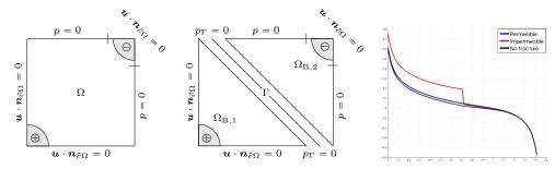
(a) Domain configurations without (left) and with (right) frac- (b) Bulk pressure over  $x_1 = ture$
