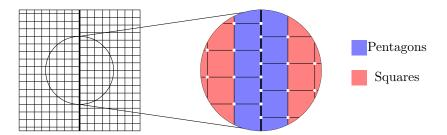
Fig. 2: Treatment of nonconforming fracture discretizations.
