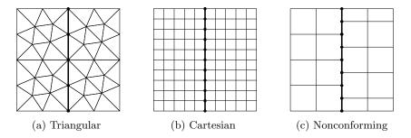
Fig. 4: Mesh families for the numerical tests
