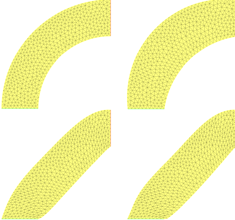
FIGURE 10. Intermediate shapes \Omega^n obtained in the bend optimization example of Section 5.1 at iterations (from left to right, top to bottom) n = 0, 5, 100 and 500.
