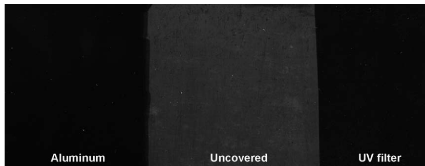
Fig. 6 Photography of the surface of a sample board after an artificial ageing for 4 weeks. From the left: the part protected by an aluminum foil (glossy and black), the uncovered part (matt and grey), and the part protected by a UV filter (slight decrease of brightness).
