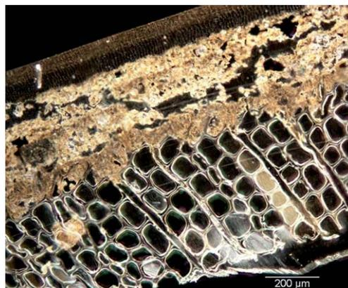
**Fig. 3** Optical image of a thin section prepared from the uncovered part of a sample board after an artificial ageing for 4 weeks. The image was obtained before the SR micro-FTIR analysis at the SMIS beamline (synchrotron Soleil).
