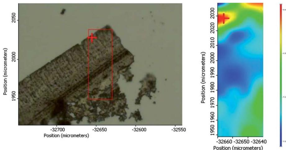
**Fig. 12** Optical image of the uncovered part of a sample board artificially aged for 4 weeks and an SR micro-FTIR image of the band at  $1716\text{ cm}^{-1}$  showing the spatial distribution of the oxidation products. A color scale from red (high intensity) to blue (low intensity) was adopted for all images. Images obtained from the microscope Continuum XL (Thermo Nicolet) at the SMIS beamline (synchrotron Soleil) and showing the  $10 \times 10\ \mu\text{m}^2$  analysed area.
