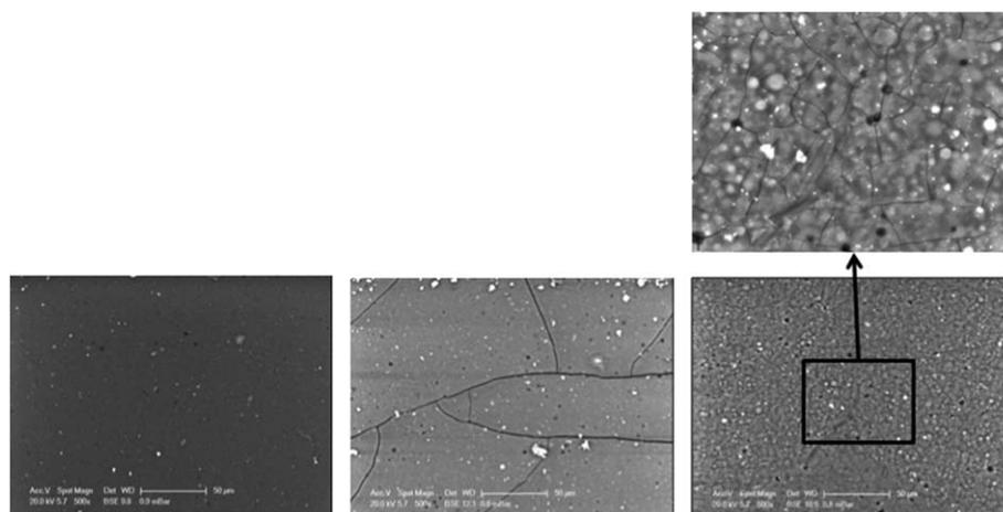
**Fig. 7** SEM images in back scattered mode of the surface of the different parts of a sample board after an artificial ageing for 4 weeks. From the left: the part protected by an aluminum foil, the part protected by a UV filter, the uncovered part with a detail showing the dense microcrack patterns (black lines) and polysaccharides (circular particles appearing in white contrast).
