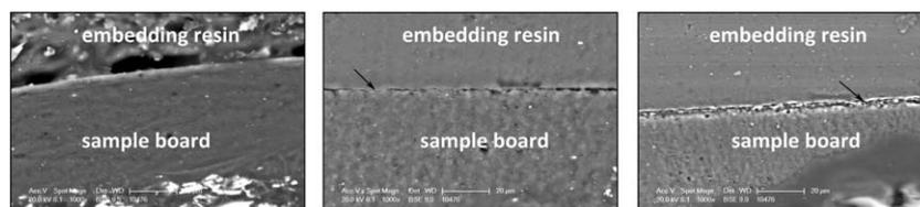
**Fig. 8** SEM images in back scattered mode of cross-sections of a sample board artificially aged for 4 weeks (magnification  $\times 1000$ ). The vertical amplitude of cracks is visible at the interface between embedding resin and sample board (reported with arrows). From the left: the part protected by an aluminum foil, the part protected by a UV filter, and the uncovered part.
