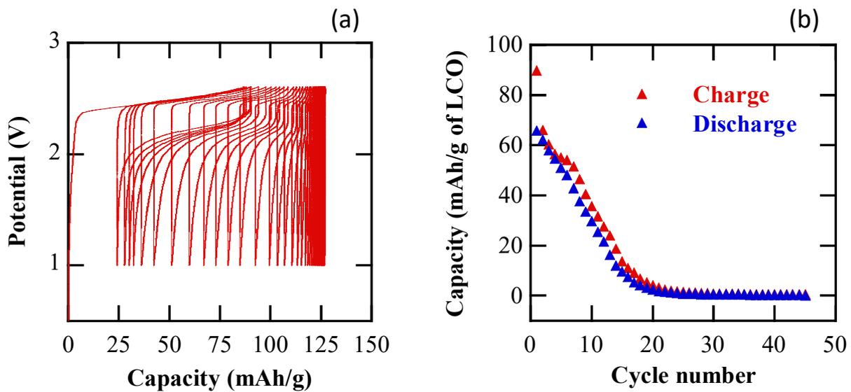
**Figure 5:** Electrochemical behaviour of a LCO / Li<sub>6</sub>PS<sub>5</sub>Cl / LTO full cell cycled between 1.0 and 2.6 V at 20°C and a C/10 rate. **a)** Charge-discharge voltage profiles. **b)** Capacity retention vs. cycle number.
