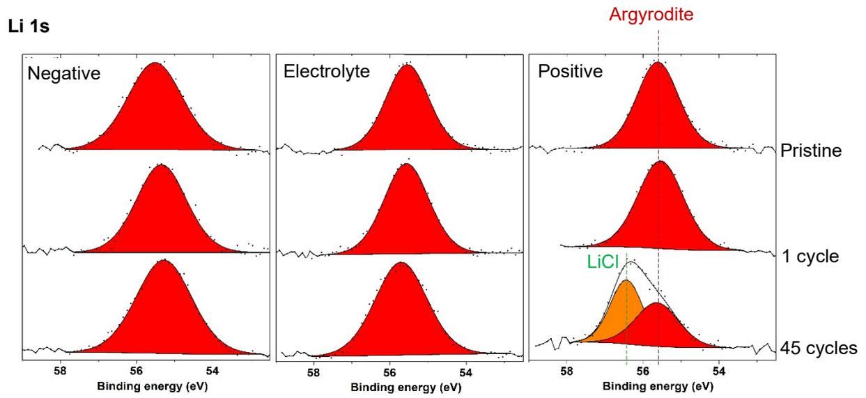
**Figure 9:** Li 1s XPS spectra of the three parts of the battery (positive and negative electrodes, solid electrolyte): before cycling (pristine), after one cycle and after 45 cycles (post-mortem).
