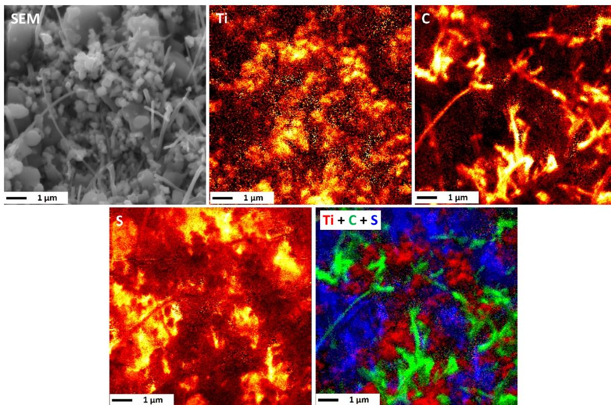
**Figure 3:** a) SEM image of the negative electrode. b), c), d) SAM mapping of the elements Ti, C and S respectively. e) SAM mapping of Ti (in red), C (in green) and S (in blue). (Bar = 1 μm)
