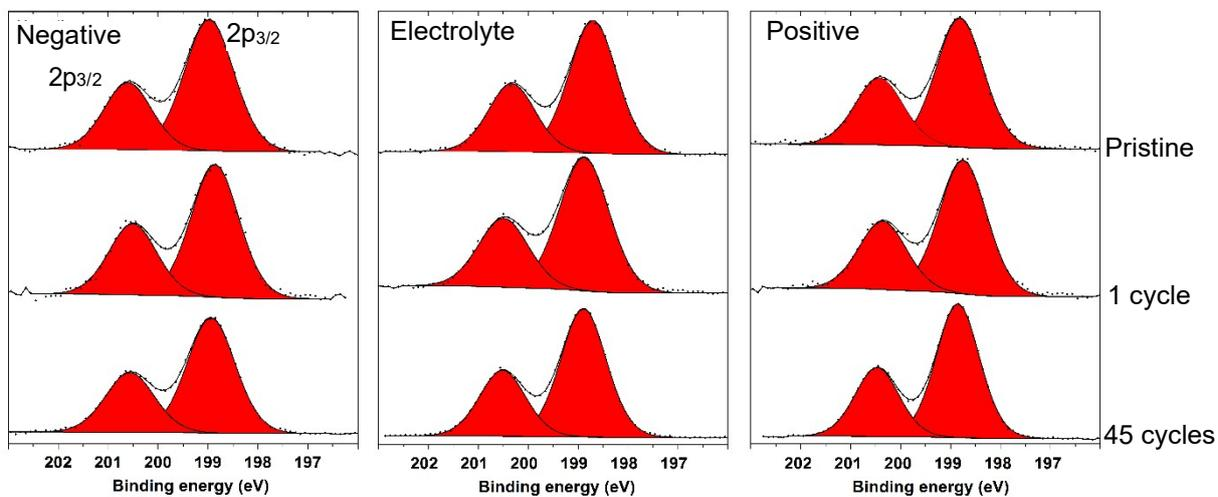
**Figure 8:** Cl 2p XPS spectra of the three parts of the LCO / Li<sub>6</sub>PS<sub>5</sub>Cl /LTO battery (positive and negative electrodes, solid electrolyte): before cycling (pristine), after one cycle and after 45 cycles (post-mortem).
