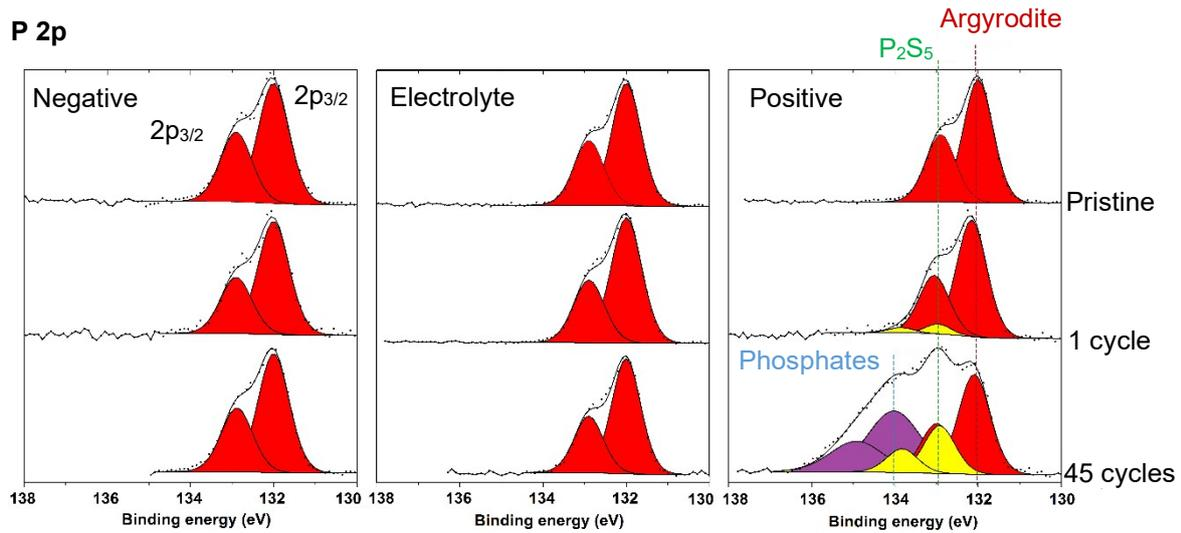
**Figure 10:** P 2p XPS spectra of the three parts of the battery (positive and negative electrodes, solid electrolyte): before cycling (pristine), after one cycle and after 45 cycles (post-mortem).
