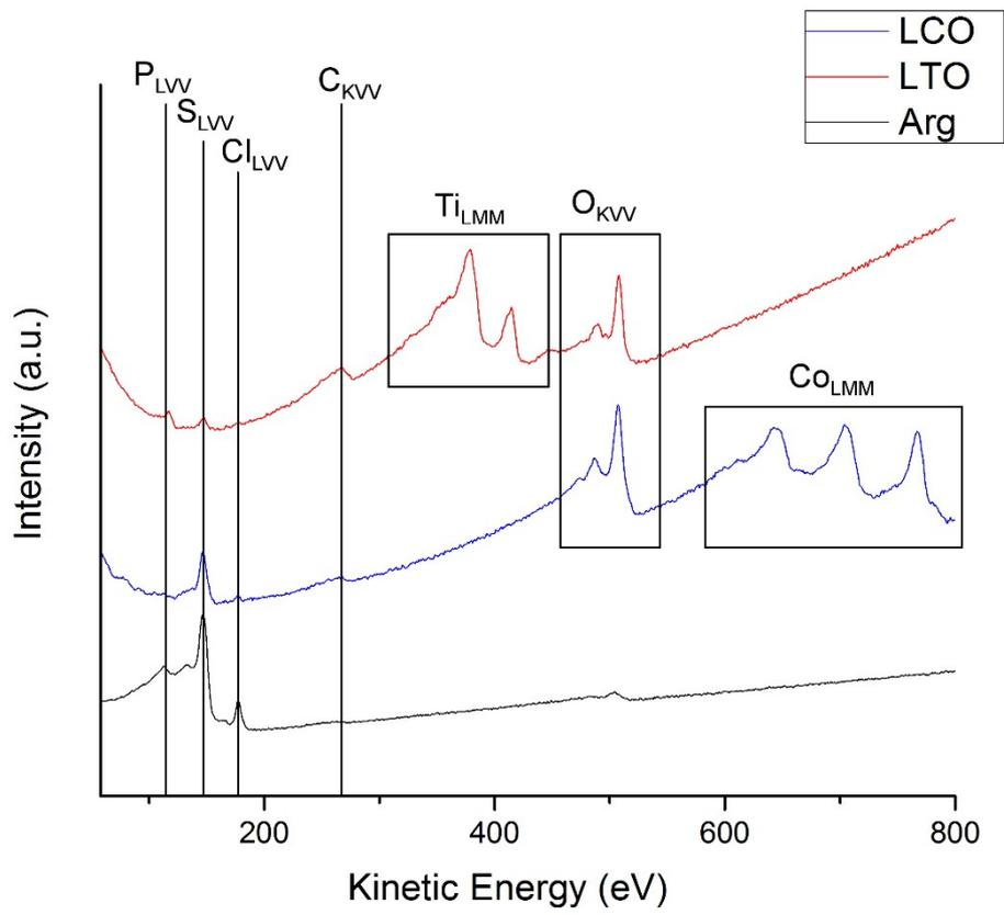
**Figure 2:** AES spectra of a LCO particle (in blue), of a LTO particle (in red) and of an argyrodite particle (in black) obtained on a cross-section of the battery.
