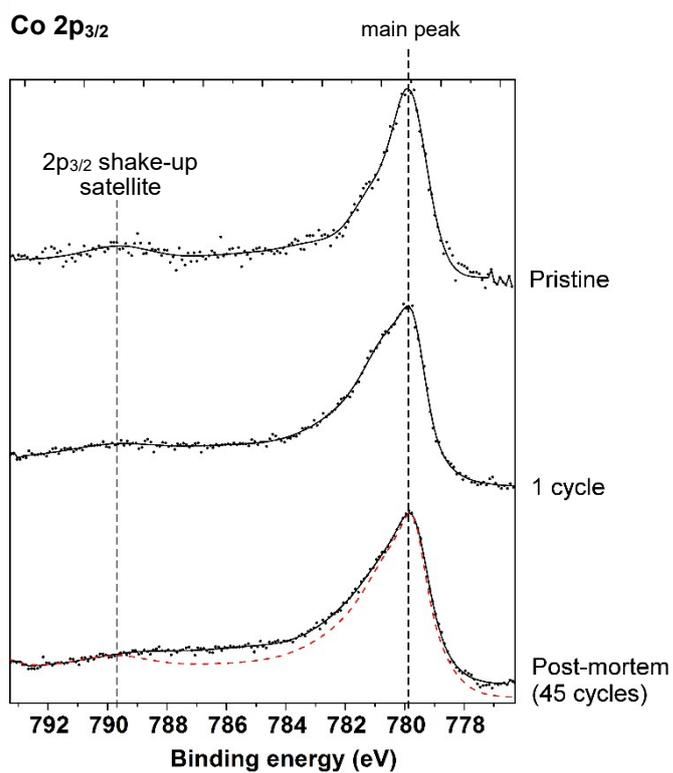
**Figure 7:** Co 2p<sub>3/2</sub> XPS spectra from the positive electrode (LCO) part of the battery, before cycling (pristine), after one cycle and after 45 cycles (post-mortem). Dashed red line corresponds to a Li<sub>x</sub>CoO<sub>2</sub> electrode (x=0.7) delithiated in a standard Li-ion cell (adapted with permission from Dahéron et al.<sup>19</sup> Copyright 2008 American Chemical Society)
