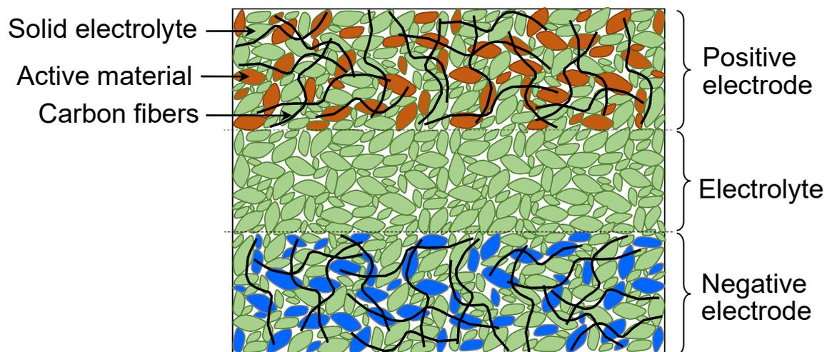
**Figure 1:** Schematic view of a cross-section of the all-solid-state battery studied in this work
