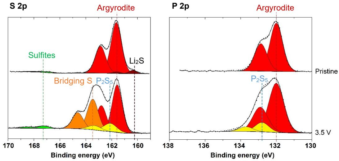
**Figure 12:** S 2p and P 2p XPS spectra of argyrodite electrode after charge of a Li<sub>6</sub>PS<sub>5</sub>Cl/Li-In half-cell up to 3.5 V. Comparison with the pristine argyrodite electrode.
