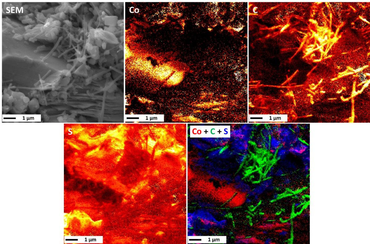
**Figure 4:** a) SEM image of the positive electrode. b), c), d) SAM mapping of the elements Co, C and S respectively. e) SAM mapping of Co (in red), C (in green) and S (in blue). (Bar = 1 $\mu$ m)
