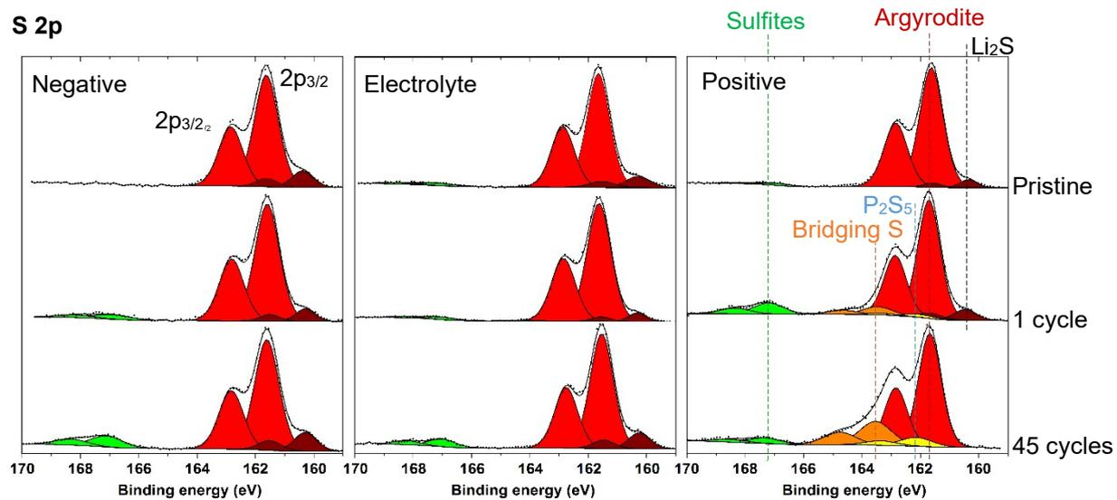
**Figure 11:** S 2p XPS spectra of the three parts of the battery (positive and negative electrodes, solid electrolyte): before cycling (pristine), after one cycle and after 45 cycles (post-mortem).
